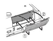
3 Loosen the lamp fixing screws.
